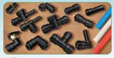
Sea Tech connectors utlize a swivel nut with NPS straight threads and a cone seal. This allows the installer to thread onto NPT, NPS, BSP and most 1/2" male threads without tools or thread sealant. Simply thread on, hand tight, for a zero-leak seal.
