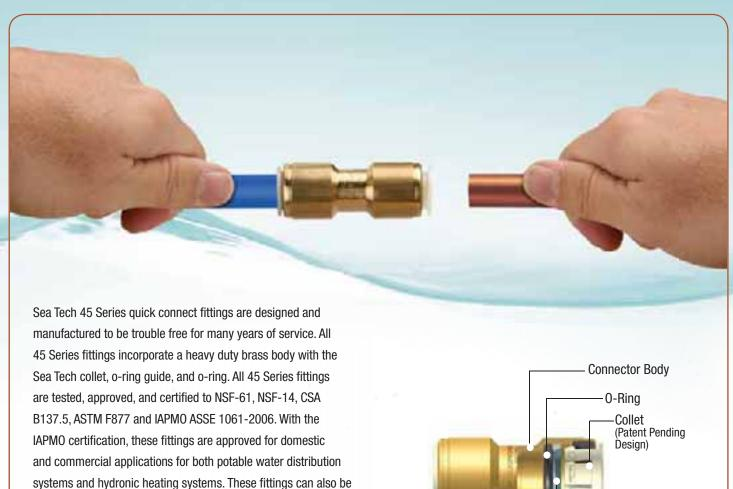
FITTINGS PERFORMANCE RATING: Operating Pressure: Vacuum to 250psi Max Temperature: 180°F @ 200psi / 75°F @ 250psi
