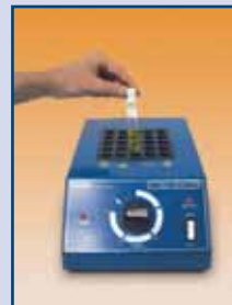
2. Place the vial in the HI 83214 reactor (sold separately) and set the timer
