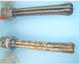
The DVGW testing was conducted during a 3 week period; one test was without Filtersorb SP3 and the other test was conducted with Filtersorb SP3. As you can see from the pictures Filtersorb SP3 worked optimally.
