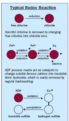
KDF process media converts hydrogen sulfide to insoluble sulfide, which can be removed by backwashing. designed for a specific need
