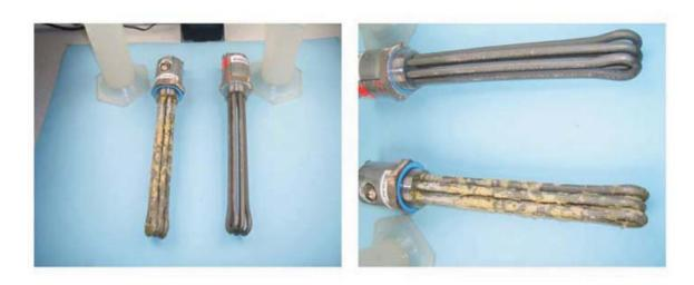
The DVGW testing was conducted during a 3 week period; one test was without Filtersorb SP3 and the other test was conducted with Filtersorb SP3. As you can see from the pictures Filtersorb SP3 worked optimally.
